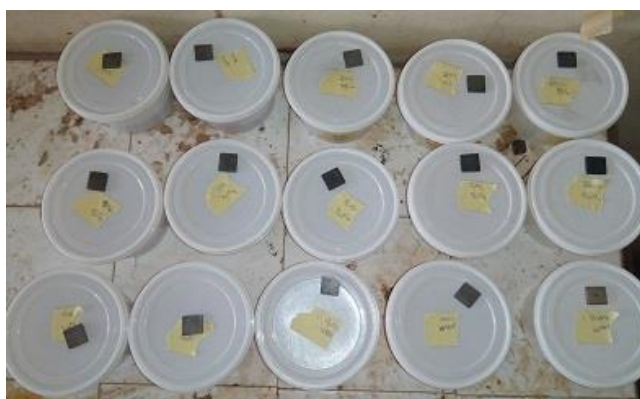
Plate 2: Experimental Set up for Gravimetric Test
